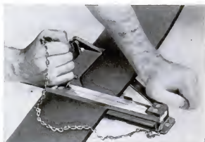
With the belt held snugly against a guide, a cutting blade is inserted through the slot
